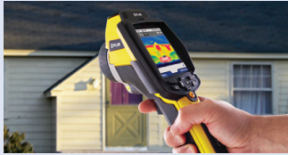
Infrared cameras quickly locate moisture related problems
