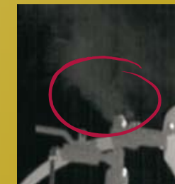
Captured gas leak from production site
